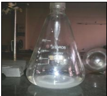
FIG. 2: VOLUMETRIC FLASK CONTAINED MSNs IN SOLUTION FORM
